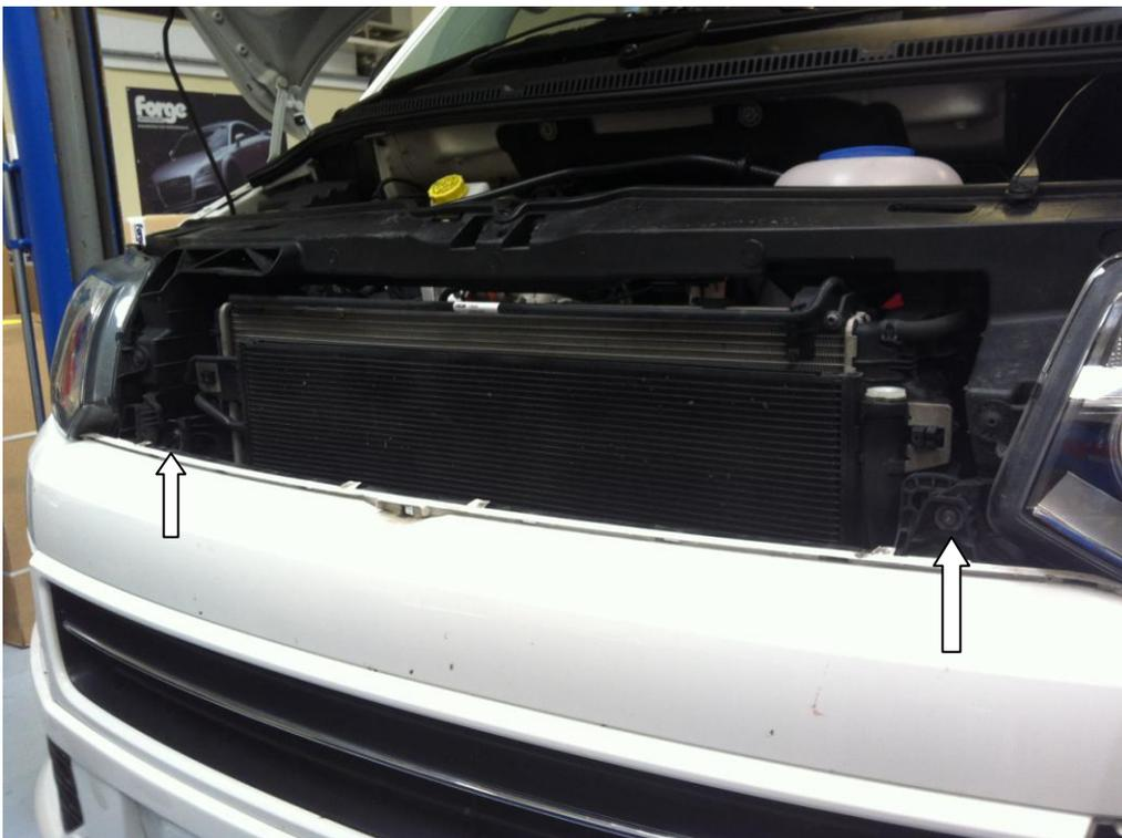
11. Now undo the T25 torx bolt situated in the middle grill on each side of the car.
