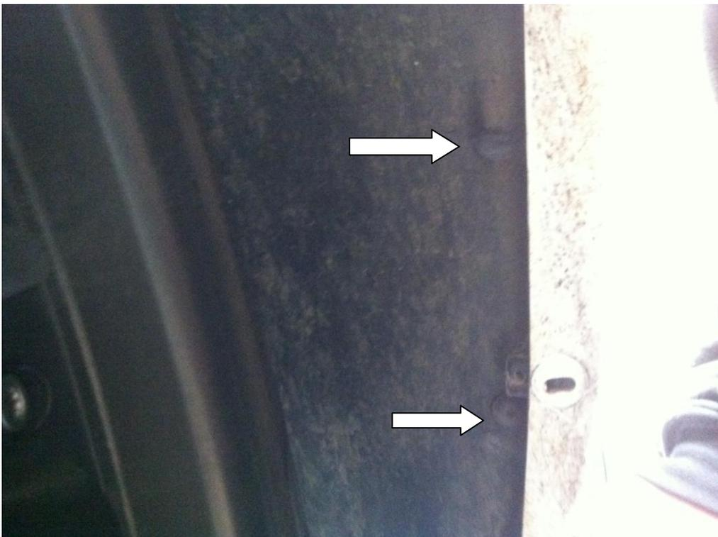
3. You will now need to peel back the wheel arch and undo the T25 torx bolt holding the bumper to the wing.
