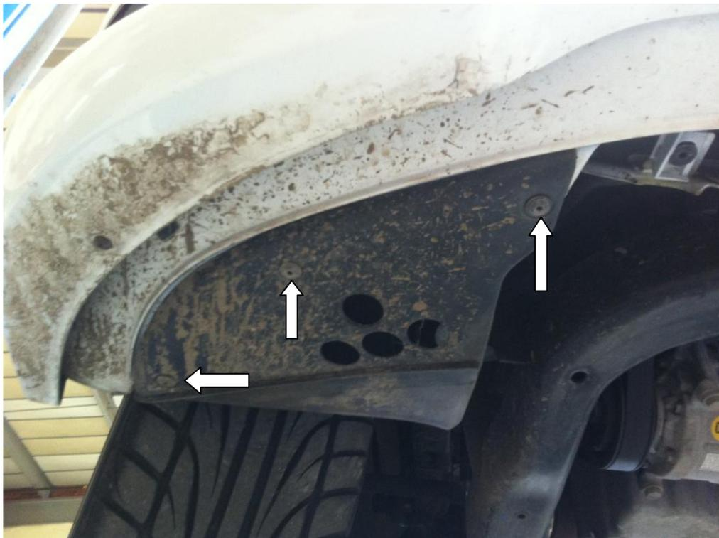
5. Undo the three T30 torx bolts holding the bottom of the bumper to the car.
