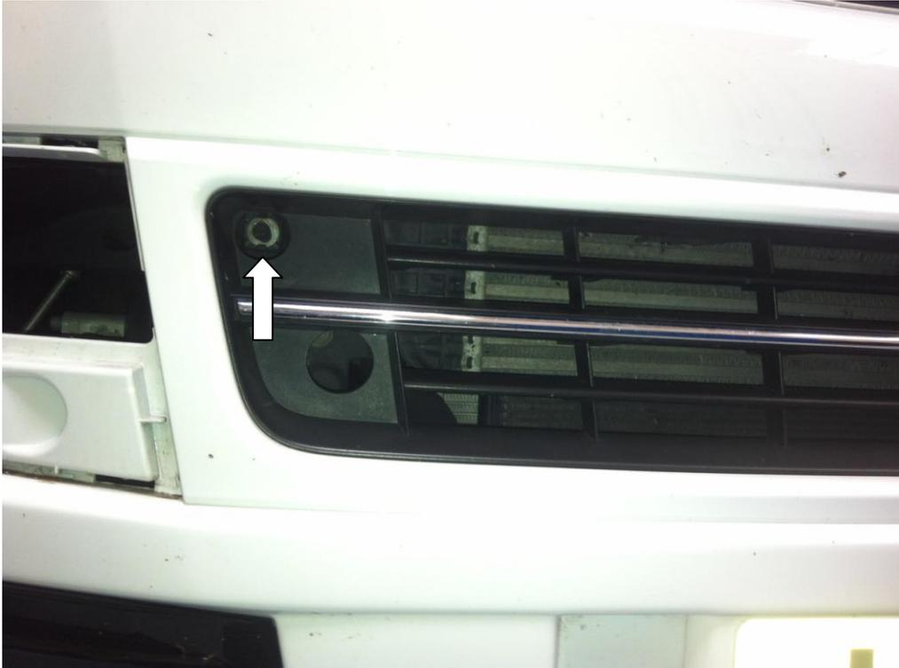
12. Now the bumper can be partly pulled away from the vehicle. Once it is slightly off you will need to remove the two plugs down on the driver side wheel arch. This is done by simply pulling back on the tabs until you here a click noise and pull apart. Place the bumper on appropriate stands as the wiring for the lights will still be attached.
