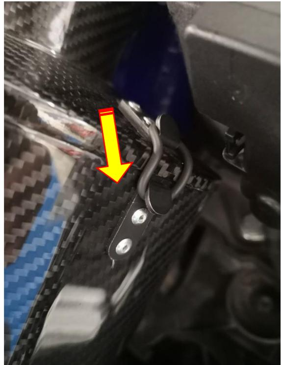
25. Using a T20 torx key screw the supplied m4 button bolts and washer into the holes at either end of the OE front airbox panel, attaching it to the rubber riv nut inside the induction kit. As you screw into it, the bolt will pull the nut inside the rubber towards you causing the rubber to create a flange inside the induction kit.
