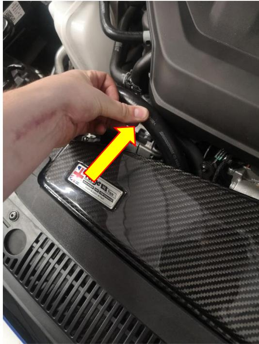
19. The next step is to prepare the filter housing element. Using the supplied 2mm thick foam strip, wrap it around the area shown below. Using a sharp knife cut the excess foam off.
