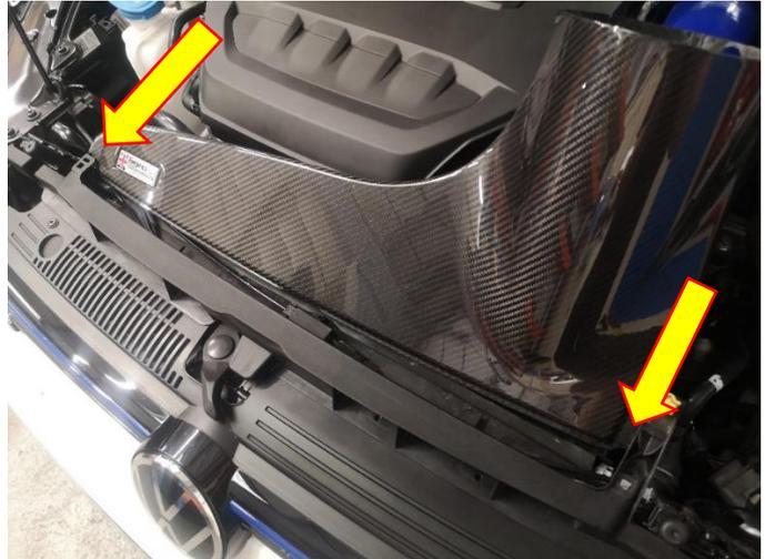
18. You will find the induction kit easier to install if you push the PAS hose shown below towards the engine to give more room to slide it into position. This hose is fine to move, push it back till it nearly touches the engine. When the induction kit is secured in place it will be positioned a good distance away from it.
