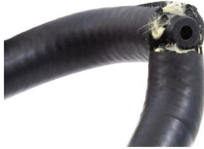
12. Insert the one-way valve into the Forge Motorsport hose in the correct orientation and push the valve fully into the hose approximately 45 mm. Do not worry how far you push it in, as when you fit the hose it will be pushed into place.
