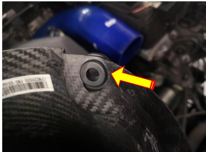
16. Pinch the flange of the rubber riv nut together and push it upwards from the underside of the slot. Repeat for the slot at either side of the induction kit.
