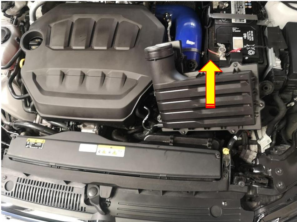
7. Press the tabs down and pull the front airbox panel towards the engine and then upwards to remove it
