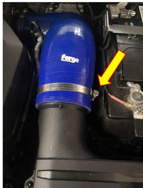
5. Pull with a sharp motion to remove the Vac line from the front right side of the engine, the other end will connect to the airbox which you can leave attached.
