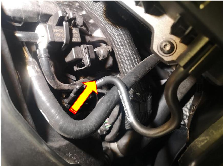
6. The airbox is located by rubber grommets on three pins. Rock the airbox left to right while pulling in an upwards motion to remove it.
