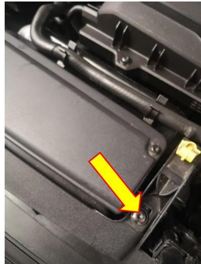
3. Unclip the coolant hose from the front airbox panel.
