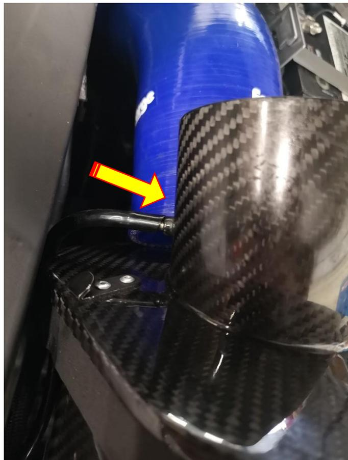
23. Using a hose clamp removal tool or a 7mm socket and suitable drive attach the OEM or Forge inlet hose to the filter housing section and tighten. Just as we mentioned for the filter, please do not overtighten the hose clamp to the carbon.
