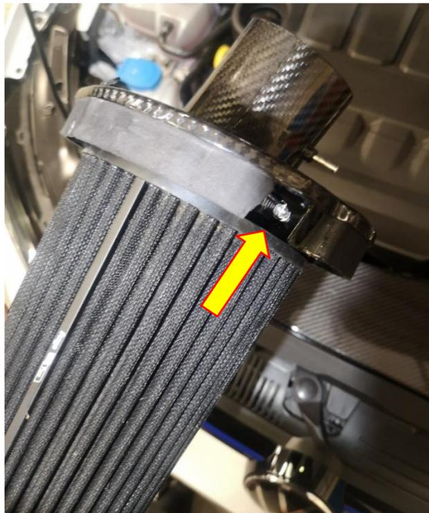
21. Tilt the rear of the large section of the induction kit towards you and push the inlet hose out the way enough to slide the filter and housing in. You'll need to locate the hole you used to tighten the filter in the filter housing with the rubber grommet on the main section of the induction kit.
