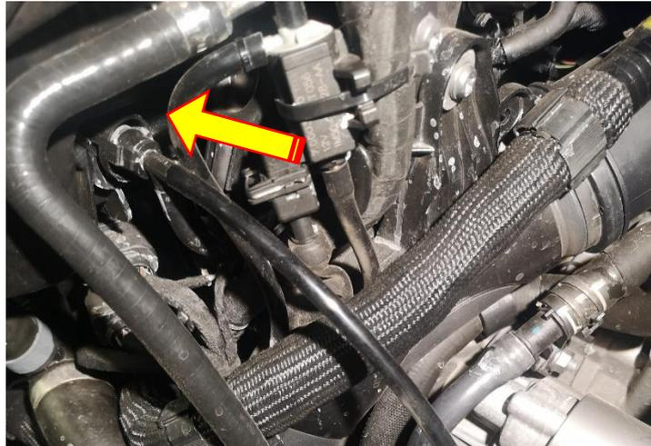
15. Install the rubber grommet in the hole on the back of the large part of the induction kit
